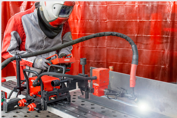
/ Radial oscillation for fillet welds.
