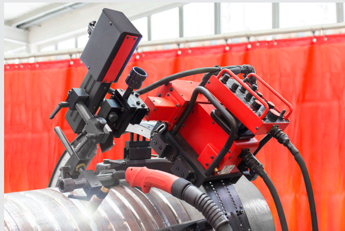
/ Linear oscillation with arc current control during orbital welding.
